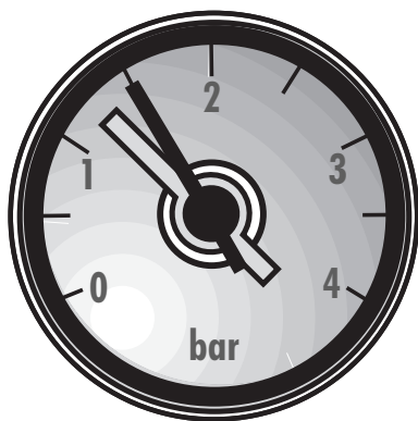
Sealed System pressure when boiler is operating
